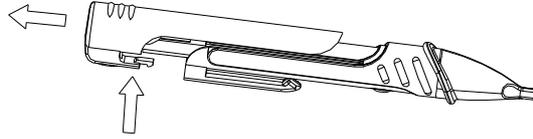
2. Insert two AAA batteries (observe polarity).
