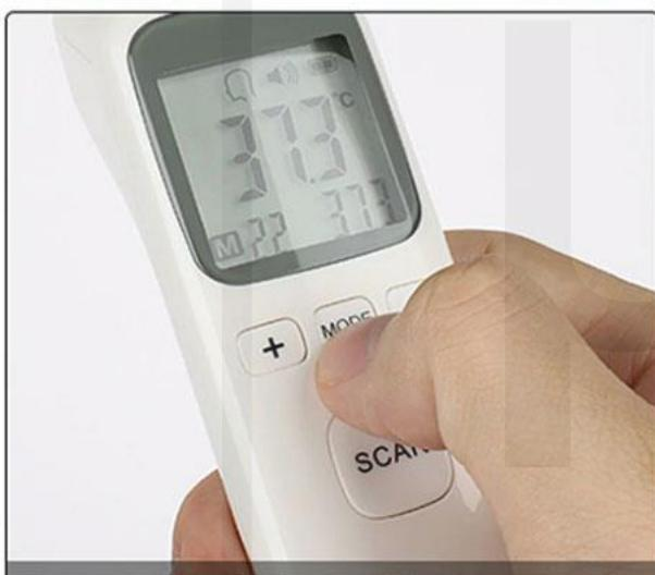
3. press "MODE", switch objec /body temperature measurement mode
