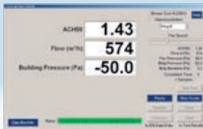
Automated BlowerDoor measurement with TECTITE Express software
