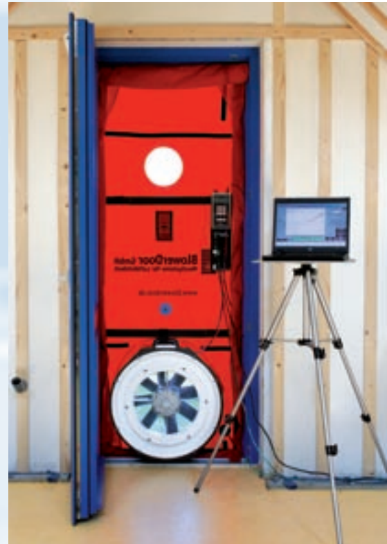
Market leader: The Minneapolis BlowerDoor with a measuring range from 19 m 3 /h to 7,200 m 3 /h
