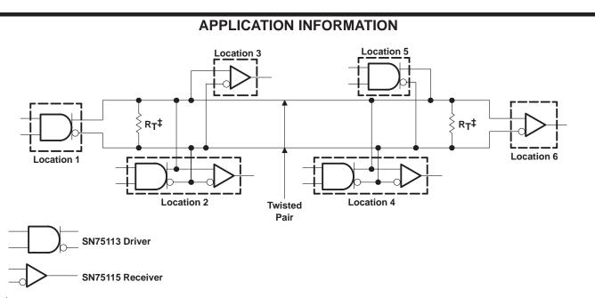
$\ddagger R_T = Z_O$ . A capacitor may be connected in series with  $R_T$  to reduce power dissipation.
