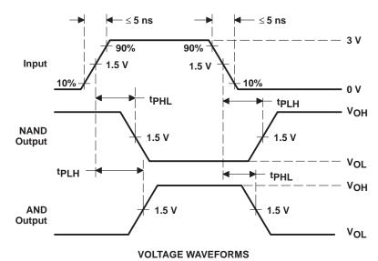
NOTES: A. The pulse generator has the following characteristics:  $Z_0 = 50 \Omega$ , PRR  $\leq 500 \text{ kHz}$ ,  $t_W = 100 \text{ ns}$ .
