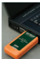
BRD10 - Optional Wireless USB Video Receiver allows user to stream live video to a PC and also can be remotely viewed via VOIP connection
