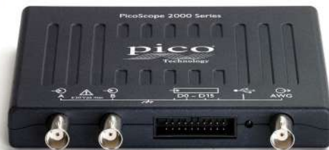
2+16-channel mixed-signal oscilloscope (MSO)
