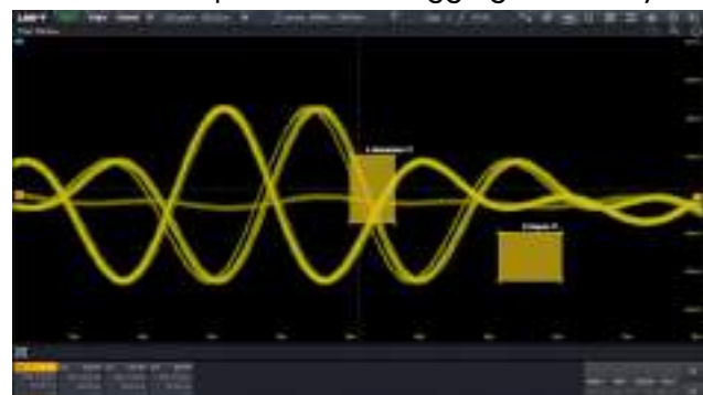
Use the zone trigger to quickly isolate unconcerned signals, quickly find key information, and there is no need to spend too much time learning advanced trigger mode
