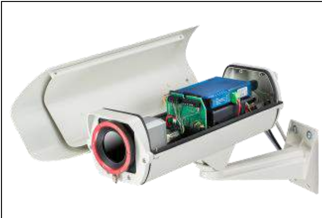
Figure 26: Outdoor protective housing for PI camera, USB server and industrial PIF
