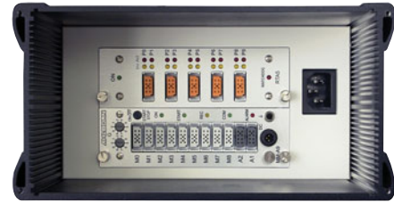
ALMEMO® 5790-2M09 IG2 View from below, floor open (Example: master measuring circuit with relay card ES5690RTA5)
