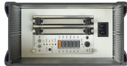
CPU system ALMEMO® 5790-2CPU IG2 View from below, floor open (Example : CPU board with 2 selector switch boards (10 ES5690MU)
