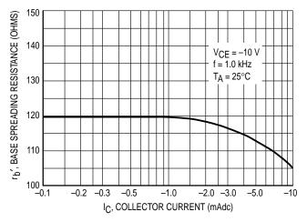
Figure 6. Base Spreading Resistance
