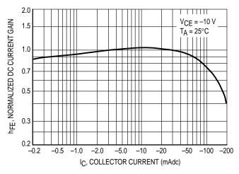
Figure 1. Normalized DC Current Gain
