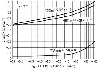
Figure 2. "Saturation" and "On" Voltages
