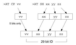
Figure 5. Setting a 29 bit CAN ID
