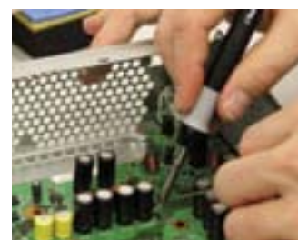
High-mass SMD soldering in hard-to-reach areas
