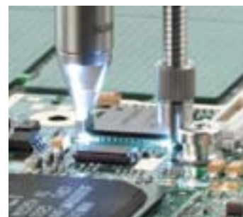
ERASCOPE inspection of components
