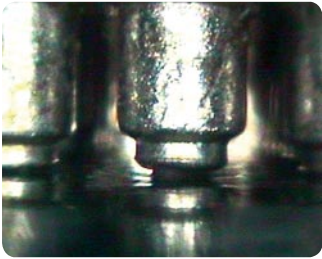
CCGA: insufficient solder
