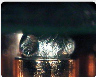
BGA: "blow hole" out gassing
