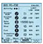
Bus Health mode allows for an analysis of the signal quality on an industrial network.
