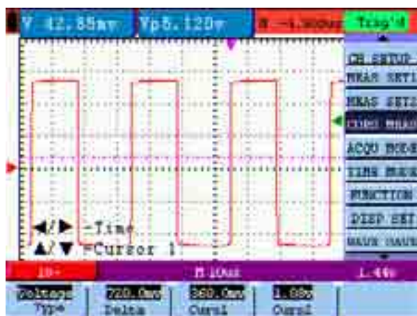
figure 45: Use the Cursor for a Voltage Measurement
