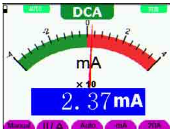
figure 24: DC Current Measurement for 400 mA
