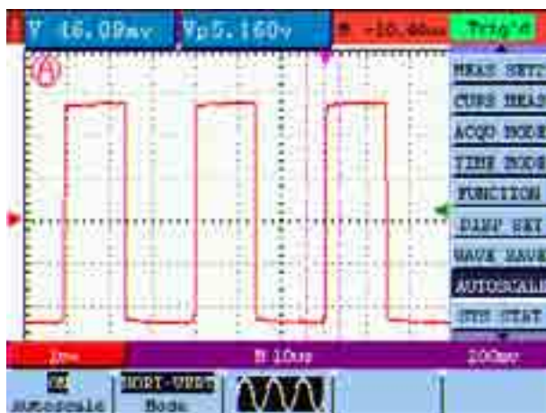
figure 47: Autoscale Horizontal- Vertical multi-period waveforms
