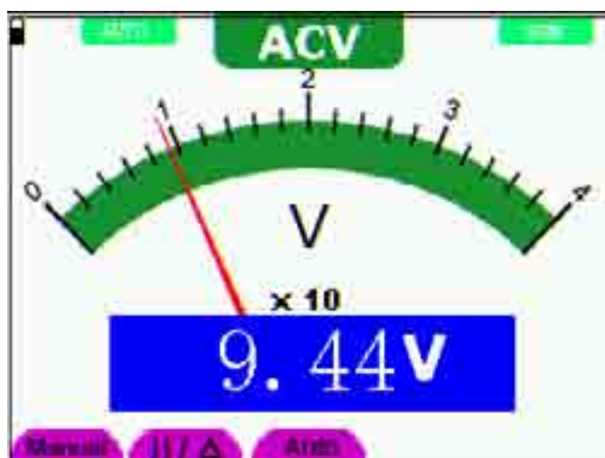
Figure 26: AC Voltage Measurement
