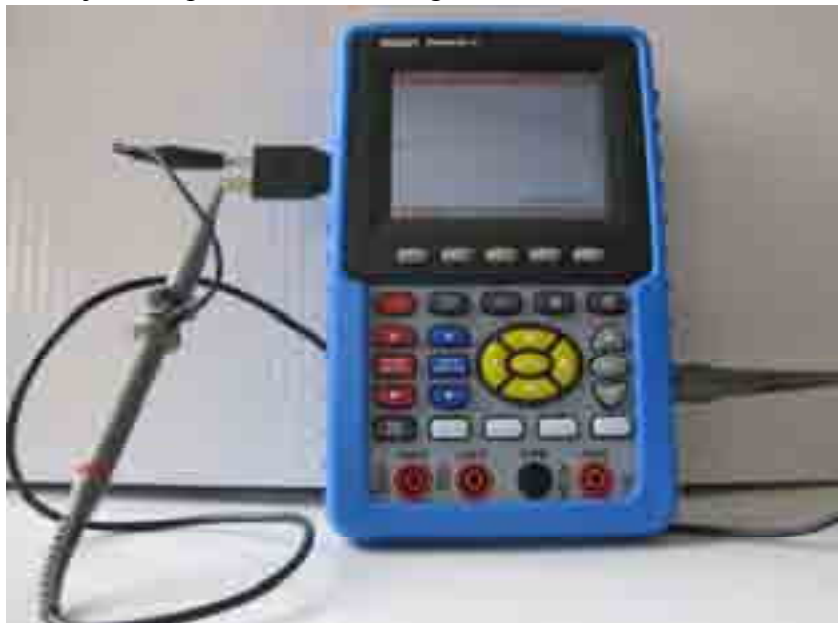
Fig.3. The connection of Square-wave test signal
