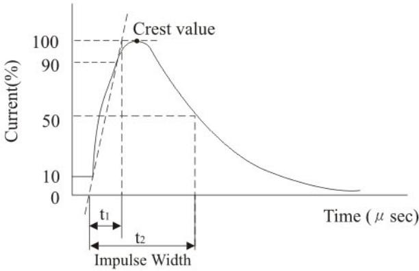
$$\begin{aligned} t_1 &= 8 \quad t_2 = 20 \quad \text{for } 8 \times 20 \mu\text{sec} \\ t_1 &= 10 \quad t_2 = 1000 \quad \text{for } 10 \times 1000 \mu\text{sec} \end{aligned}$$
