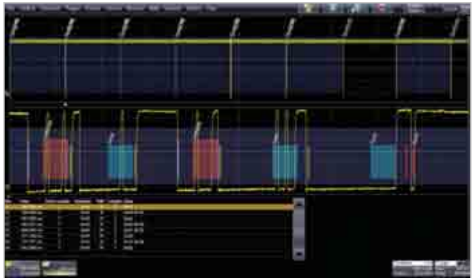
I 2 C decoding package with intuitive color decoding and table view allows quick location of 0x42 address.
