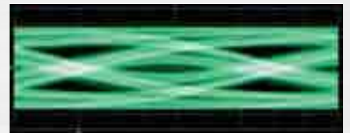
As the serial data rate increases, the attenuation in the backplane “closes” the eye diagram at the input to the receiver.
