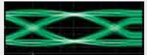
By using Eye Doctor II to apply serial data channel emulation to correct for backplane emulation, then using Eye Doctor to apply receiver equalization to mimic functionality of the hardware receiver, we can understand whether the signal as received by the receiver has acceptable jitter performance or not.
