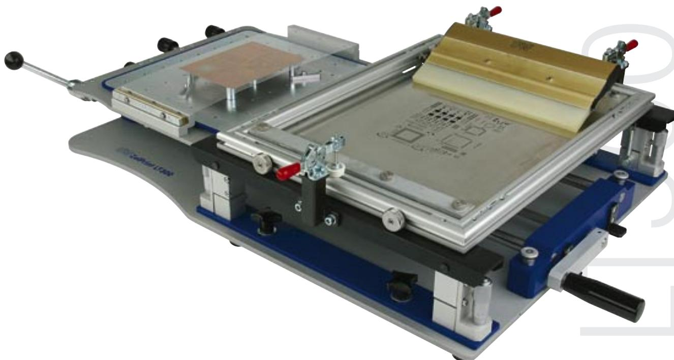
The LPKF ZelPrint LT300 is a precision manual stencil printer. This tabletop model can be used for prototypes and for small batches of fine pitch SMT boards. On-contact fine-pitch printing, precise vertical separation between stencil and PCB, and slow snap-off provides superb printing results. This unique solution allows printing of 0.3 mm (12 mil) pitch (ultra-fine-pitch area).
