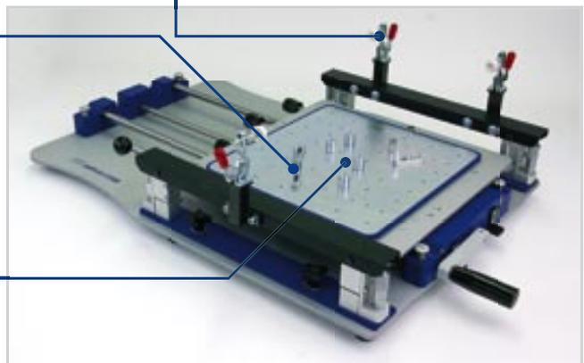
**Plastic stencil for rapid PCB prototyping**
