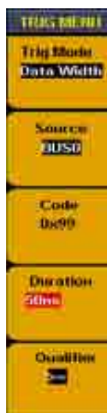
Fig.5-64: Duration trigger menu
