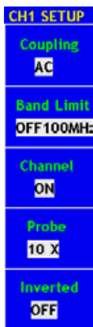
Fig. 5-1 Channel Setting Menu
