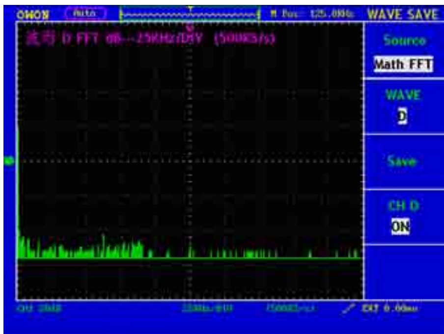
Fig.5-39 FFT wave Saving
