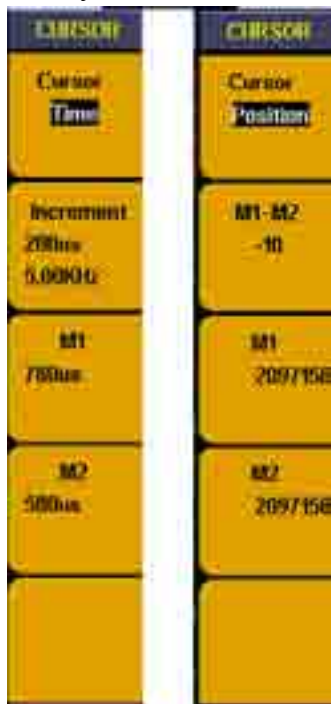
Fig.5-79: Cursor measurement menu
