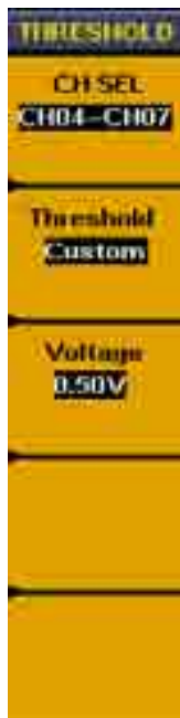
Fig.5-66: Threshold setting menu
