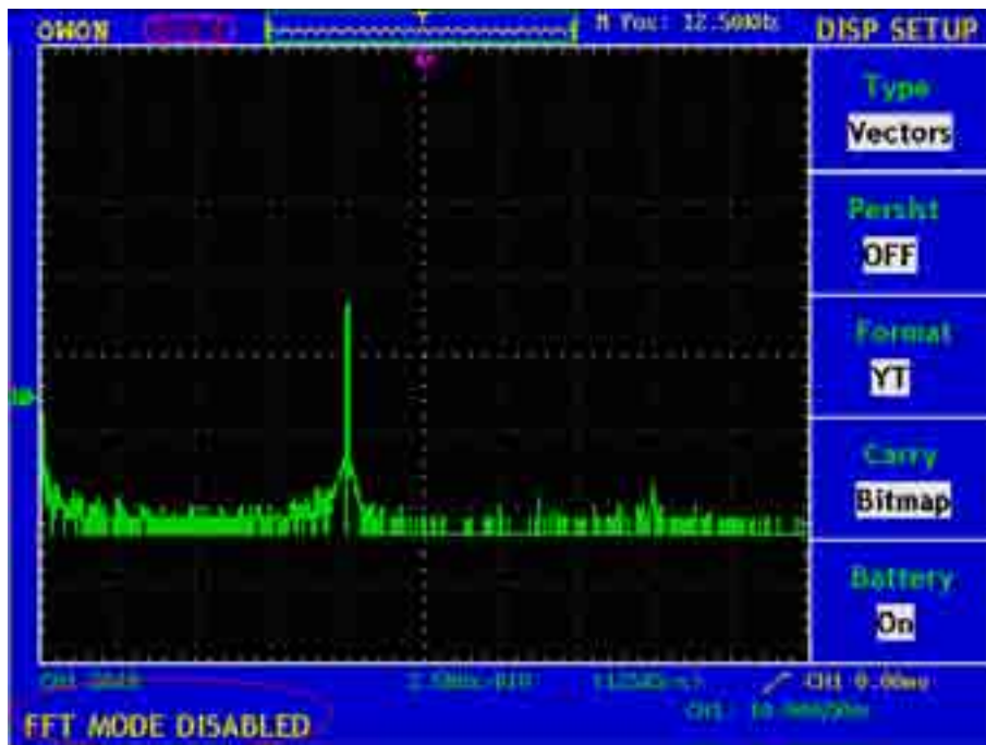
Fig.5-36 FFT mode XY Format Disable
