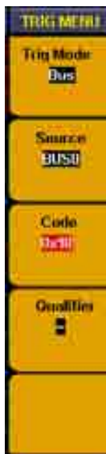
Fig.5-56: Bus trigger menu
