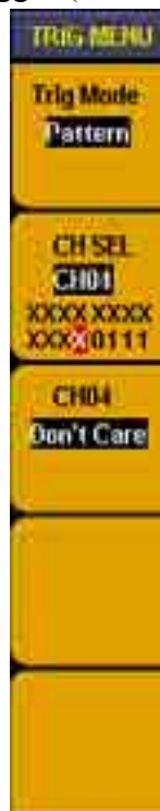
Fig.5-58: Pattern trigger menu
