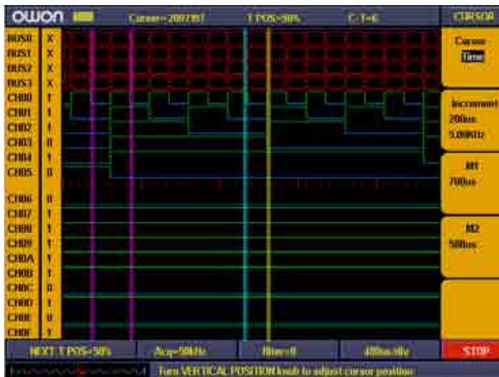
Fig.5-80: Cursor time measurement
