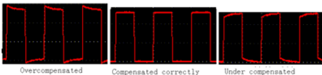
Fig. 4-5 Displayed Wave Forms of the Probe Compensation
